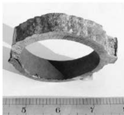
Fig. 12.19 Cross section of an overlaid waterwall tube showing alloy 625 overlay after 16 years of service in a RDF unit in Lawrence, MA. Courtesy of Welding Services Inc.
