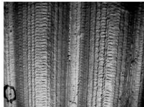
Fig. 12.21 Close-up view of alloy 625 overlay on the waterwall of another RDF boiler after 10 years of service. Shown in the photograph are two tubes and a membrane. Courtesy of Welding Services Inc.
