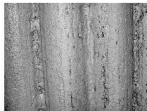
Fig. 12.22 Pitting attack is the common mode of corrosion of alloy 625 weld overlay on the waterwall. Shown in the photograph are three tubes and three membranes.
