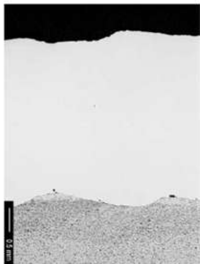
Fig. 12.20 Optical micrograph showing the cross section of the alloy 625 overlay of an overlaid waterwall sample (Fig. 12.19) obtained from a RDF boiler (Lawrence, MA) after 16 years of service. Micrograph also shows the fusion boundary and substrate carbon steel. Courtesy of Welding Services Inc.
