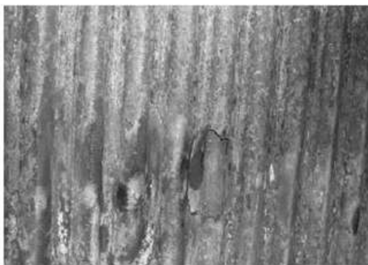
Fig. 12.4 Carbon steel waterwall suffering blown tubes due to high wastage rates resulting in significant tube-wall thinning after 8 months of service in a WTE boiler. Courtesy of Welding Services Inc.
